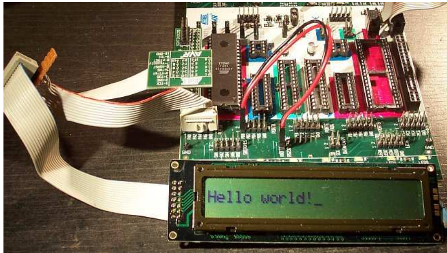
Figure 5: Wiring of the STK500
